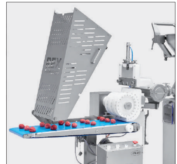
High performance thanks to multi-row form rollers
