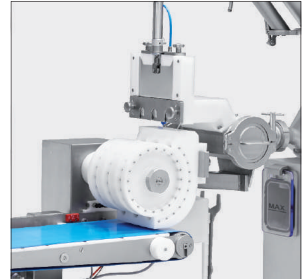
High performance thanks to multi-row form rollers
