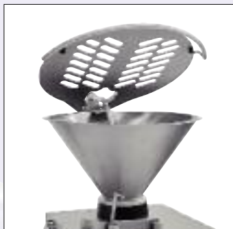
casing holding device, fixed for natural casings
