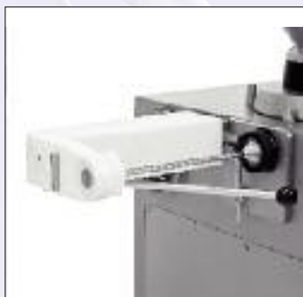
casing holding device, fixed for natural casings
